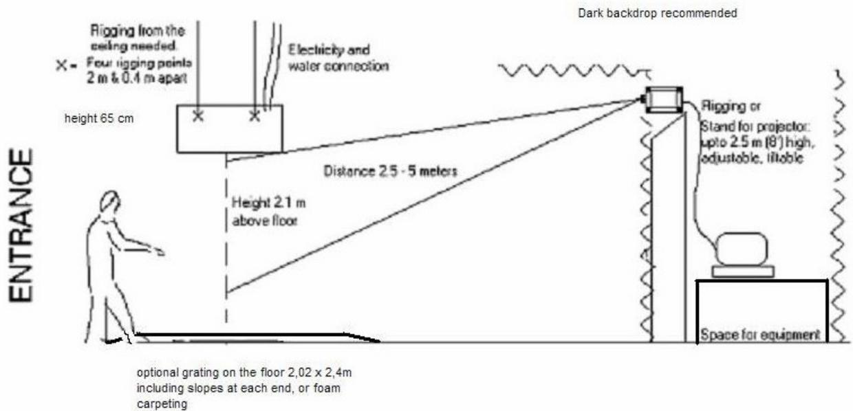
Rigging from the ceiling or from a ground support
